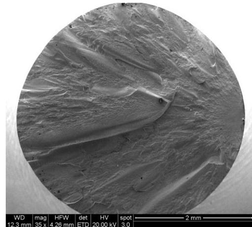
Fig.4: Fatigue fracture surface of hardmetal at about 10E+9 cycles (UFTH Stage 1)
