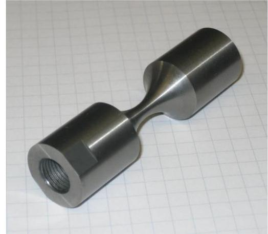
Fig.2: Hardmetal fatigue test bar for ultrasonic resonance testing (fixing by thread at one end)
