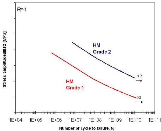
Fig.1: S-N graphs of two different hardmetal grades (UFTH Stage 1)
