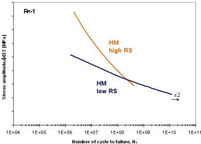
Fig.3: S-N graphs of HM grade 2 with different RS
