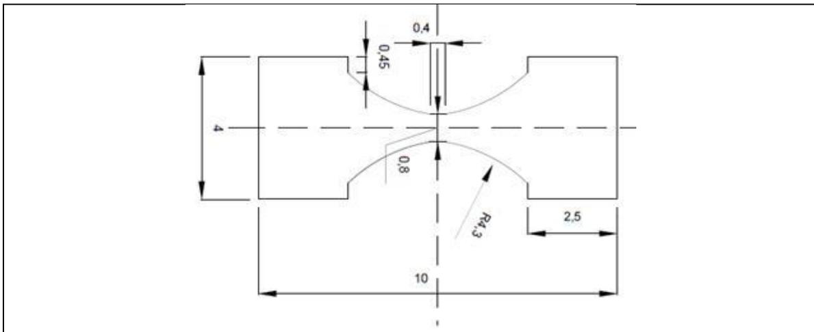
Figure 1. Sketch of the tensile specimen geometry (dimensions are in mm). Thickness: 1mm
