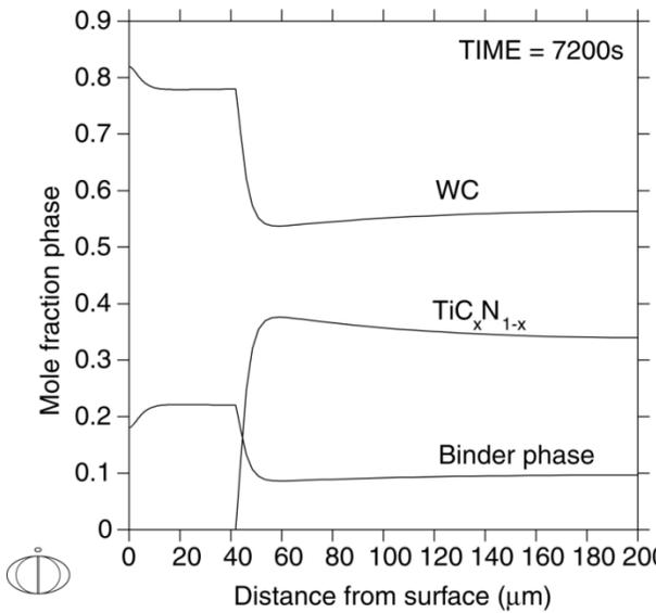
Figure 1. Simulation of gradient zone using the same mobilities for all elements.
