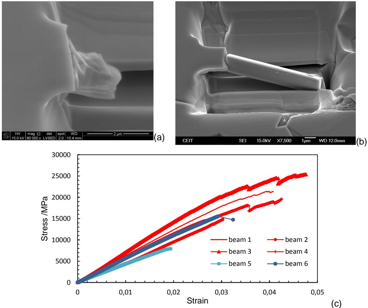
Figure 2. SEM images of cantilevers milled on a coarse grain WC-Co hardmetal with (a) CSL2 interface and (b) no CSL2 interface close to the fixed end after bending test. (c) Corresponding stress-strain data for cantilever beam bending with in red CSL2 interface and in blue no CSL2 interface. Note data for beams 1, 2 & 4 is incomplete as they touched the substrate before complete fracture.
