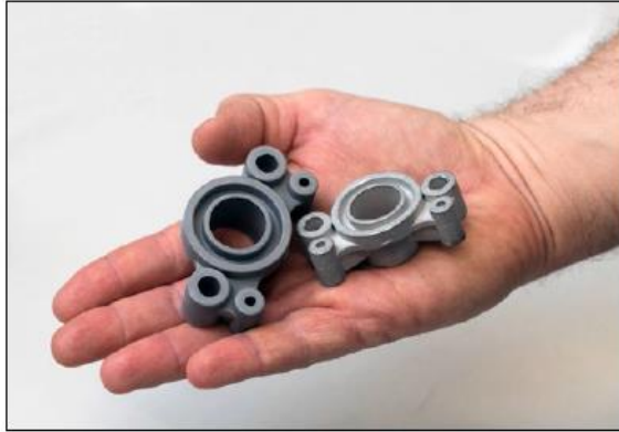
A green aluminium MIM part, left, and the sintered part on the right
